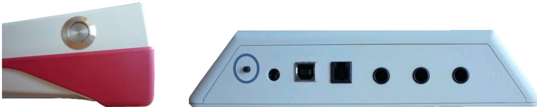
Figure 2: On/off switch for handheld (left) and desktop device (right, marked with blue circle)
