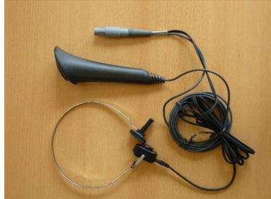
*Fig. 15: Patient response switch combined with bone conductor*
