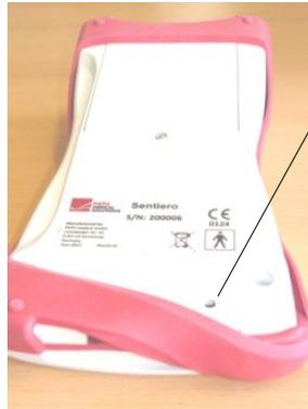
Push the reset button below the rubber casing on the back side of the device with a pen. Afterwards the device can be turned on with the on switch.
