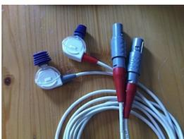
*Fig. 5: OAE probe (TE: grey and DP: red) with red tension relief*
