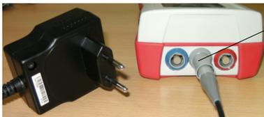
Fig. 13: Power supply and charging cable with grey tension relief
