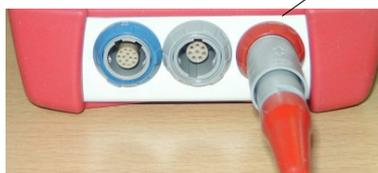
Ear probe (for OAE measurements) plug with red tension relief.
