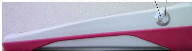
Fig. 2: On / off switch on the right-hand side of the device; special functionality during MAGIC and SUN module.
