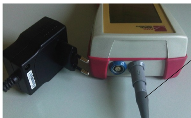
Fig. 10: Power supply and charging cable with grey tension relief
