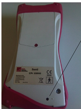
Fig. 3: Black reset button on the back side of the device below the red rubber casing
