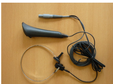
Fig. 12: Patient response switch combined with bone conductor
